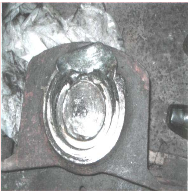
Figure 2. The aspect of the fracture zone in the extremity of the wheelset (lubrication boxes)
