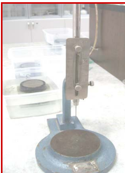
Figure 9. Vicat apparatus for determination of water for the normal consistence paste
