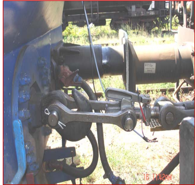
Figure 2 Drawing hook with strain gauges
