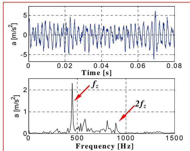
Fig. 2 Time runs and vibration signal spectra of the toothed gears in rolling stand drives in rolling time a – gear in general good dynamic condition (cage k4), b – gear classified for repair (cage k12).
