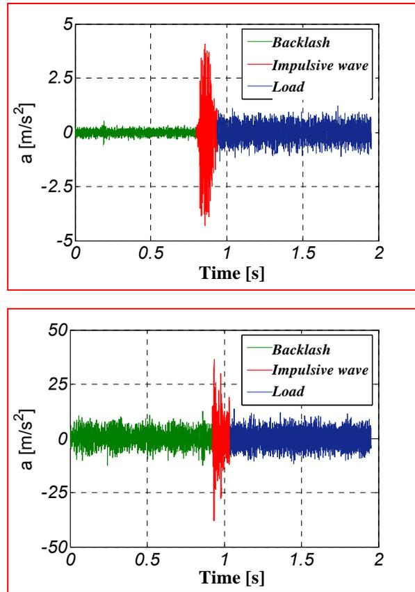
Fig. 1 Registered vibration signals of toothed gears of the rolling stand drives, a – gear in general good dynamic condition (cage k4), b – gear classified for repair (cage k12)
