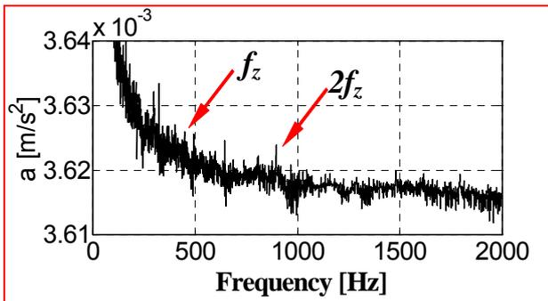
Fig. 5 Product spectra of toothed gears vibration signals in rolling stand drives in rolling time a – gear in general good dynamic condition (cage k4), b – gear classified for repair (cage k12).
