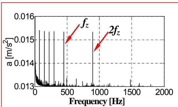
Fig. 4 Poly-harmonic spectra of toothed gears vibration signals in rolling stand drives in rolling time a – gear in general good dynamic condition (cage k4), b – gear classified for repair (cage k12).
