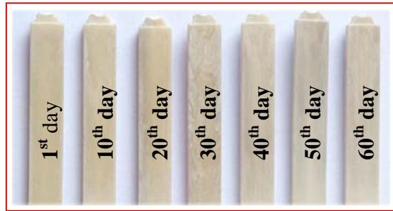
Fig. 9 Specimens biodegradation in NEUTRAL area
