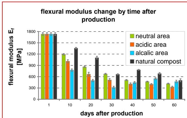
Fig. 2 Flexural modulus results
