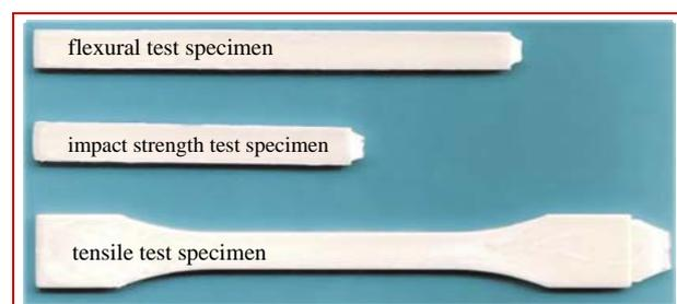
Fig. 1 Mechanical properties test specimens
