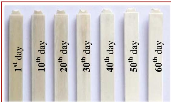
Fig. 7 Specimens biodegradation in ACIDIC/ALCALIC area.
