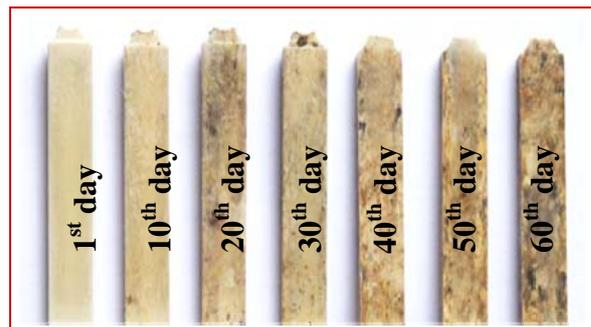
Fig. 11 Specimens biodegradation in NATURE COMPOST
