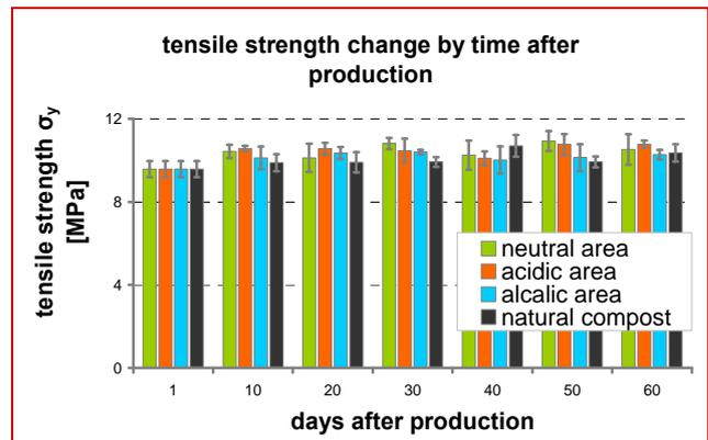
Fig. 4 Tensile strength results
