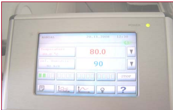
Figure 1. Control and monitoring panel for climatic chamber Vötsch, type VC 7060
