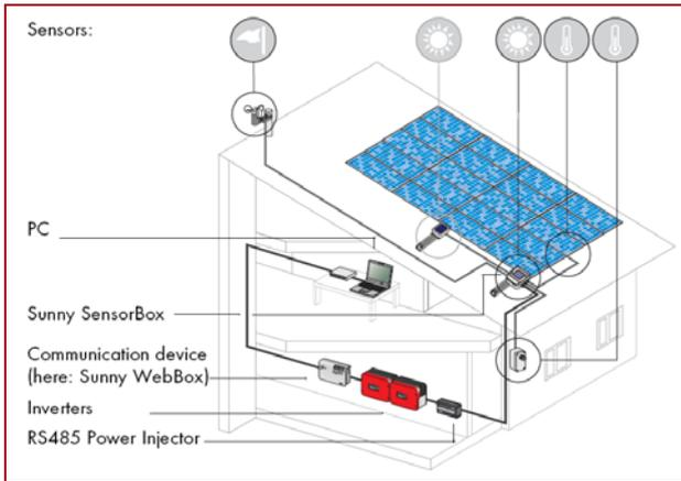
Figure 1 Complete scheme, photovoltaic and monitoring system
