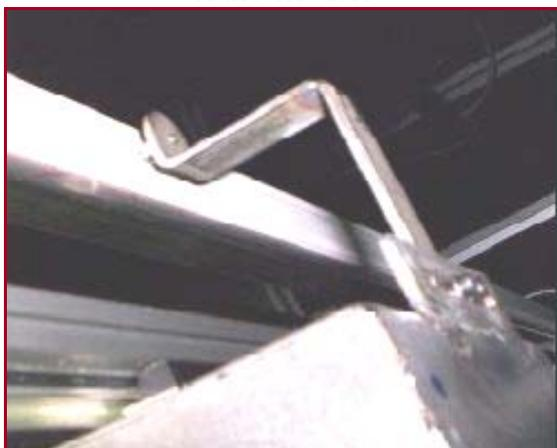
Figure 7: Scanning of the position of elevator cabin with means of a magnet moving along the sensor plinth
