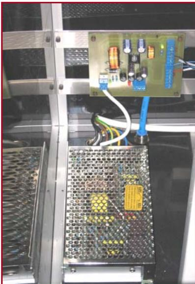
Figure 6: Realization of power supply of the elevator
