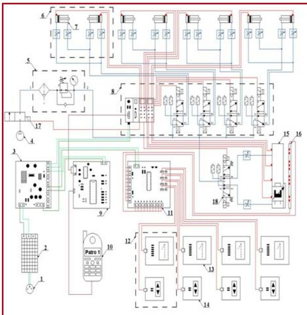
Figure 3: Scheme of controlling the elevator model (Legend: red – electrical signals, blue – pneumatic signals brown – RS - 232, green – power supply)
