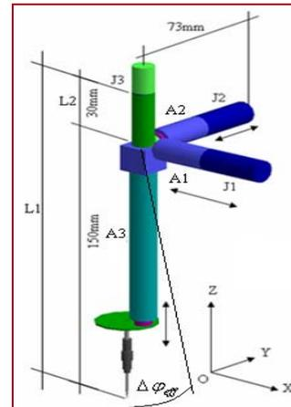
Figure 8. Virtual model of microrobot
