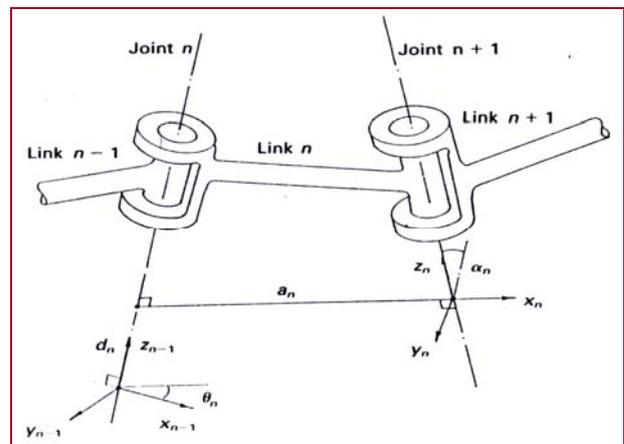
Figure 6. Link coordinate frame allocation
