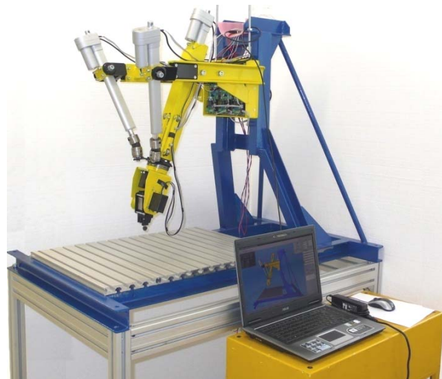
Figure 9 - Small-scale CNC machine tool builds on trivariant hybrid kinematic structure
