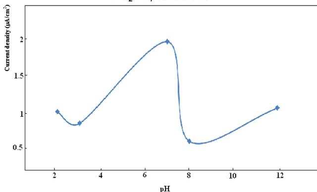
Figure 7. Effect of the pH on square wave voltammogram peak height of 10 mg/L Pb<sup>2+</sup> in 0.1M Na<sub>2</sub>SO<sub>4</sub>, accumulation time: 15 min
