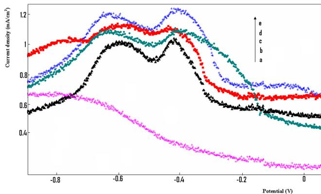
Figure 10. Square wave voltammograms in 0.1M Na<sub>2</sub>SO<sub>4</sub> under the optimized conditions at CP-S electrode of lead (II): a- 0 mg/L, b- 5 mg/L, c- 8 mg/L, d- 10 mg/L and e- 20 mg/L.
