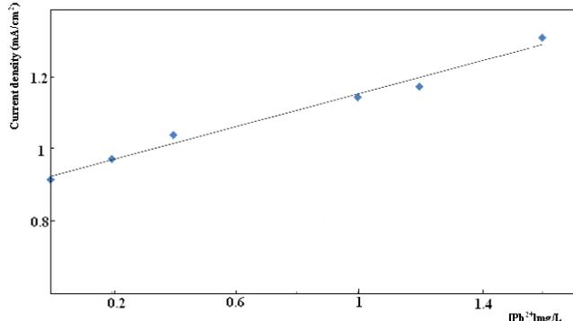
Figure 8. Influence of concentration of lead on the peaks intensity at CP-S electrode under the optimized conditions
