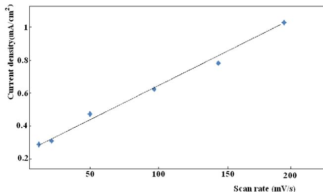
Figure 5. Influence of the scan rate on the oxidation peak intensity for 10 mg/L Pb<sup>2+</sup> (pH 7.0) in 0.1M Na<sub>2</sub>SO<sub>4</sub>, preconcentration time 15 min.
