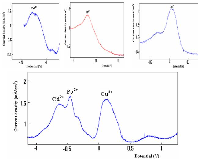
Figure 9. Cyclic voltammograms of 10 mg/L lead, 10 mg/L cadmium and 10 mg/L copper at CP-S electrode, pH 7.0, 15 min of preconcentration time in 0.1M Na<sub>2</sub>SO<sub>4</sub>.
