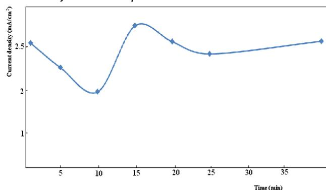
Figure 6. Influence of preconcentration time on the oxidation peak of 10 mg/L lead pH 7.0 on square wave voltammograms at CP-S electrode in 0.1M Na<sub>2</sub>SO<sub>4</sub> solutions
