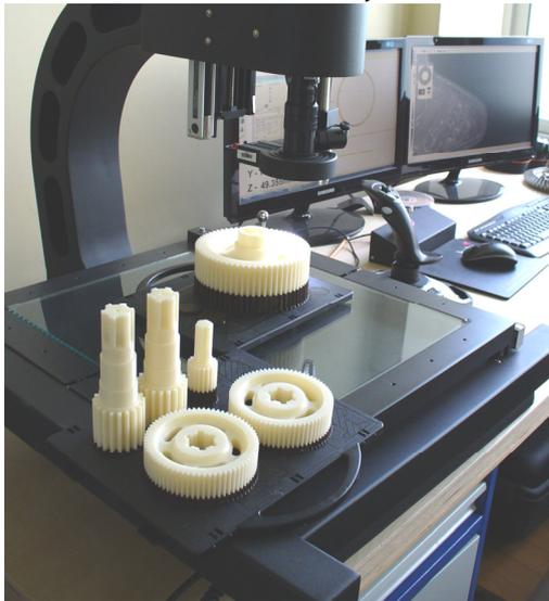
Figure 3. The coordinate measuring system - BATY VENTURE
