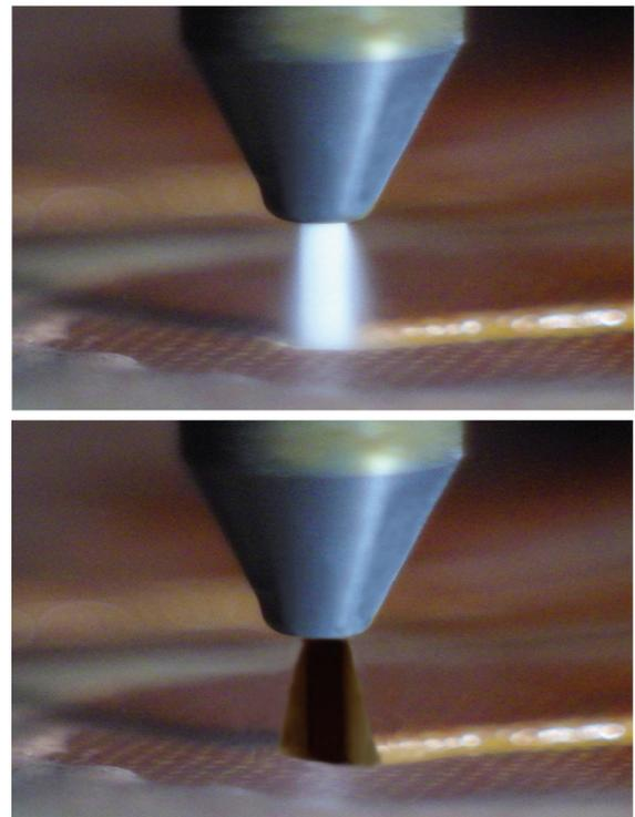
Figure 3: Hydroerosive jet surrounded by water mist
