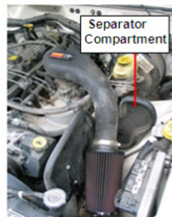
Figure 2. Installing filters in separator compartments
