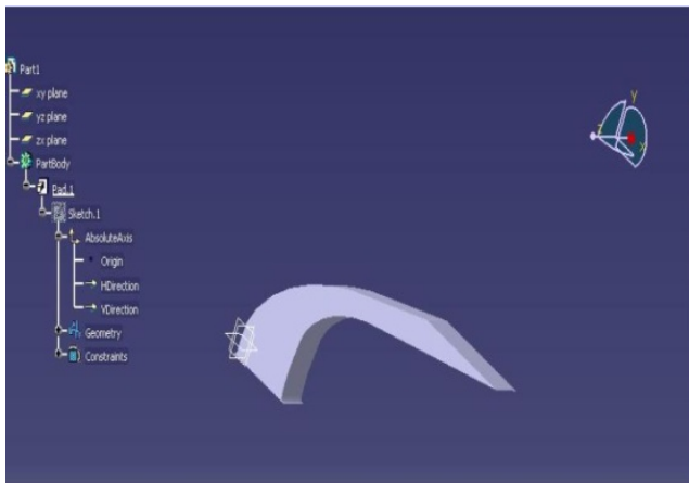
Figure 2: Geometry of rectangular bent nozzle
