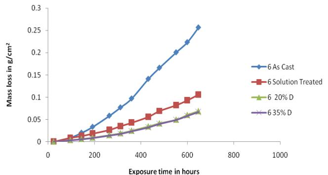
Figure 5(a): Variation of mass loss against exposure time of 6% alumina reinforced composite samples
