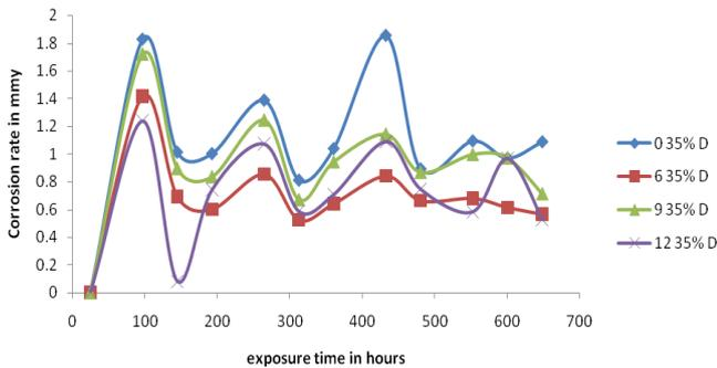
Figure 4(b): Variation of Corrosion rate against exposure time of alloy and composites subjected to 35% cold deformation plus solution treated
