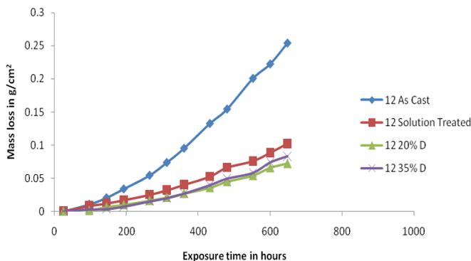
Figure 7(a): Variation of mass loss against exposure time of 12% alumina reinforced composite samples
