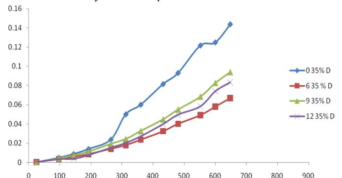
Figure 4(a): Variation of mass loss against exposure time of alloy and composites subjected to 35% deformation plus solution treatment.
