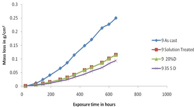
Figure 6(a): Variation of mass loss against exposure time of 9% alumina reinforced composite samples
