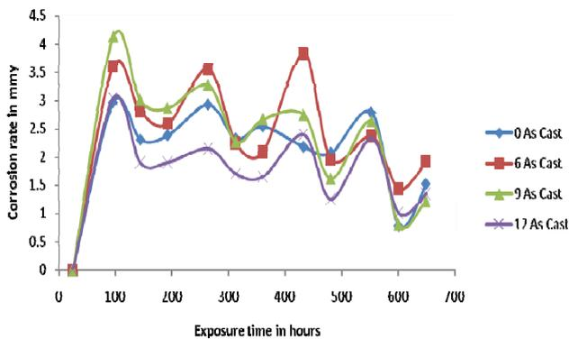
Figure 1(b): Variation of Corrosion rate against exposure time of as cast alloy and composites
