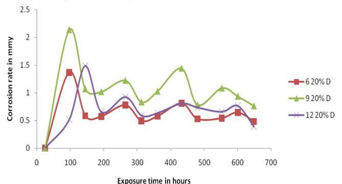
Figure 3(b): Variation of Corrosion rate against exposure time of alloy and composites subjected to 20% cold deformation plus solution treated
