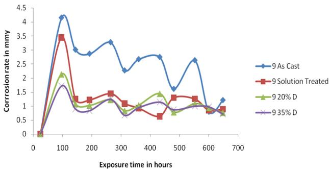
Figure 6(b): Variation of corrosion rate against exposure time of 9% alumina reinforced composite samples
