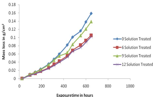
Figure 2(a): Variation of mass loss against exposure time of solution treated alloy and composites.
