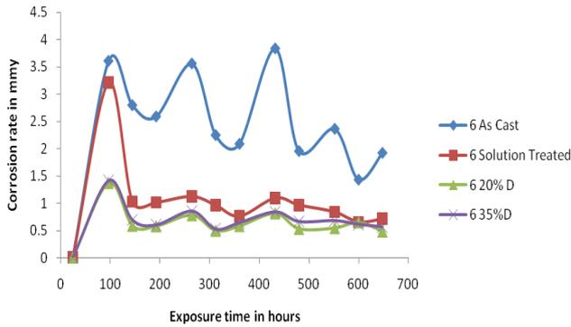
Figure 5(b): Variation of corrosion rate against exposure time of 6% alumina reinforced composite samples
