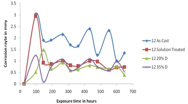
Figure 7(b): Variation of corrosion rate against exposure time of 12% alumina reinforced composite samples
