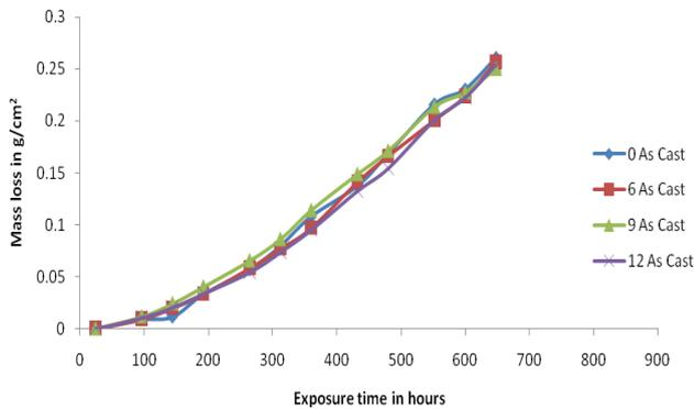
Figure 1(a): Variation of mass loss against exposure time for as cast alloy and composites
