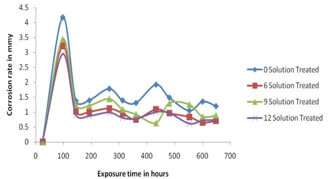
Figure 2(b): Variation of corrosion rate against exposure time of solution treated alloy and composites
