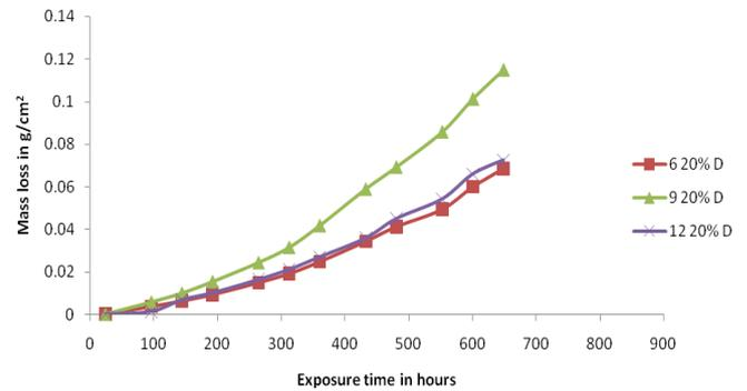
Figure 3(a): Variation of mass loss against exposure time of alloy and composites subjected to 20% deformation plus solution treatment.
