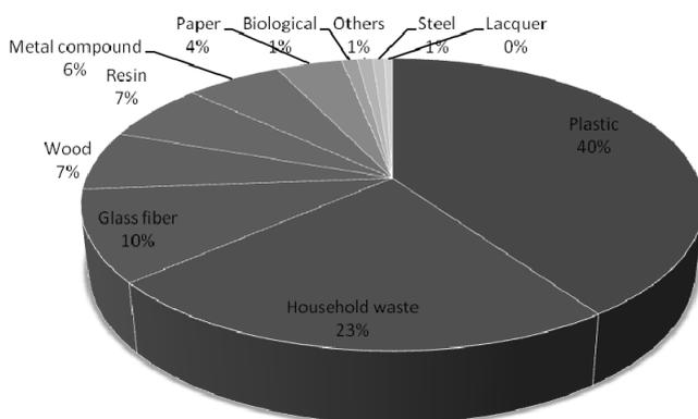
Figure 4 – Waste generated to produce 180 rotor blades [16]
