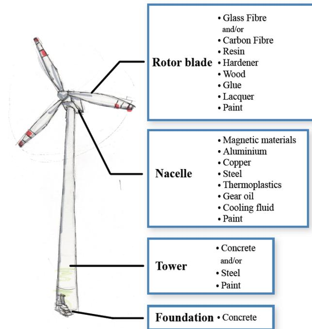
Figure 1 – Materials involved in each part of the final wind turbine [14, 15, 16]
