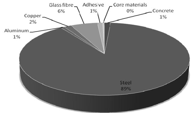
Figure 2 – Distribution of raw materials in wind turbines without foundations (1.5 MW) [17]
