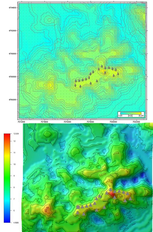
Figure 1. Mean wind speed fields simulated in WAsP (left) and WindSim (right)
