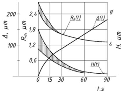
Figure 1. Pre-honing:  $t$  machining time changes depending on the important characteristics.
