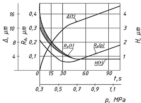
Figure 2. Finishing or fine - honing:  $t$  machining time and  $p$  tool pressure function changes and important characteristics. Data from the  $t$  - dependence curves:  $v_t = 40$  m/min;  $v_a = 12$  m/min;  $p = 0,5$  MPa; Data from the  $p$  - dependence curves:  $t = 60$  s, other data as described above.
