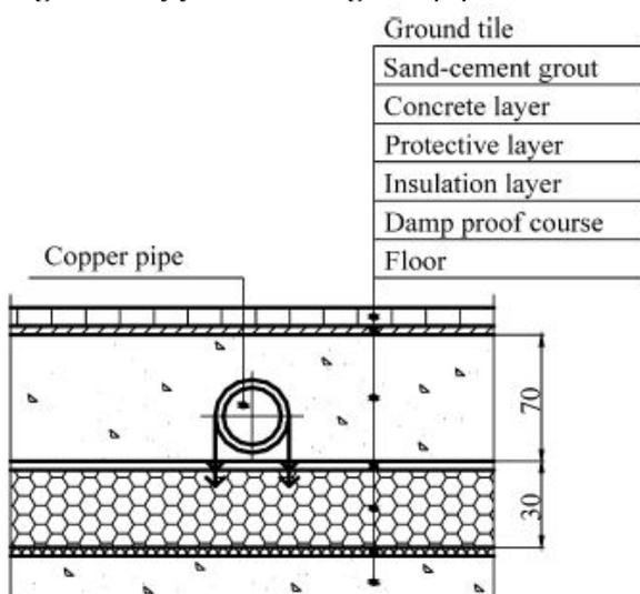
Figure 2. Arrangement of floor heating coil pipe
