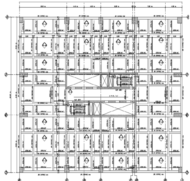
Fig. 4 Paneled beams slab plan system
