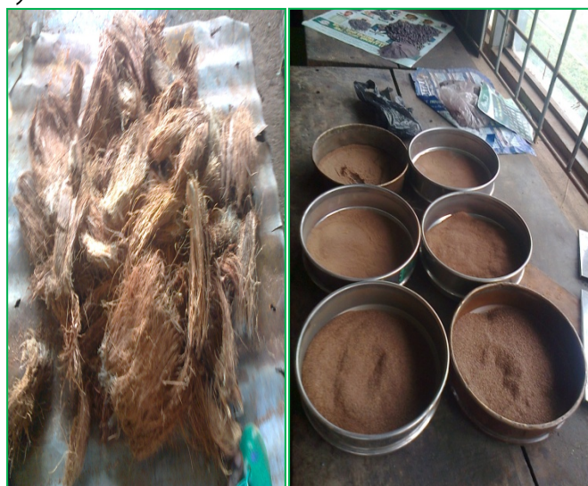
Figure 2. Sun drying of coconut coir (left) and extracted coconut coir particle (right)
