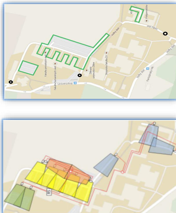
Figure 1. The distribution of parking spaces in University campus, input-output terminals are marked (left), a design of deployed cameras showing the coverage of sectors (right)
