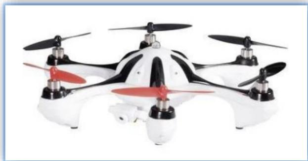
Figure 1. Hexa-rotor microcopter used for the experiments
