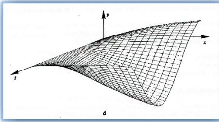
**Figure 3.** Axial vibration in  $y$ - $x$ - $t$  space.
