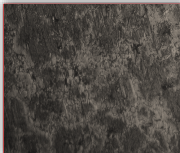
Plate 2: Microstructure of sample B 60 percent by volume of PEG (after quenching operation) – 200X
