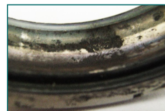
Figure 5. Fretting corrosion on the outside rolling track of ball bearing [11]
