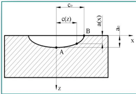
Figure 1. Surface crack idealization
