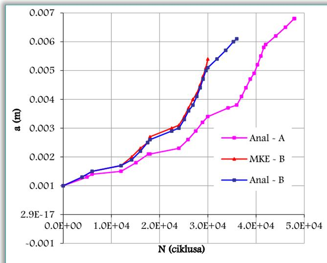
Figure 4. Surface crack growth under load spectra
