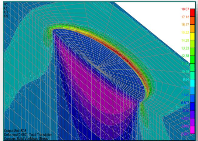
Figure 2. Detail finite element model of semi-elliptical crack
