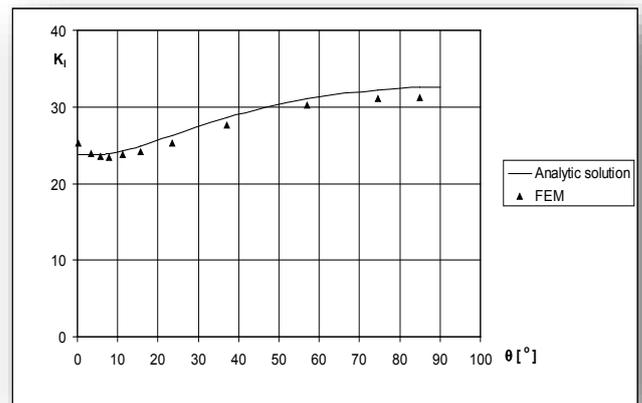
Figure 3. Comparisons between analytic and FE results for SIF calculations
