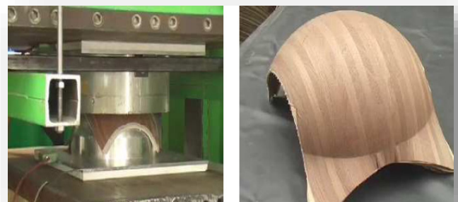
Figure 3. The process of making 3D plywood with male and female template [8]
