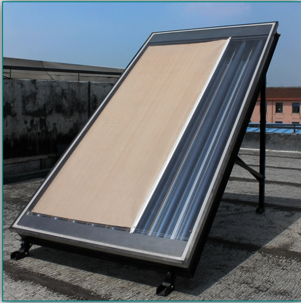
Figure 1. Automatic shading system DESIGNING PROCESS OF THE PHOTOVOLTAIC SOLAR WATER HEATER SYSTEM (PV-SWHS)
