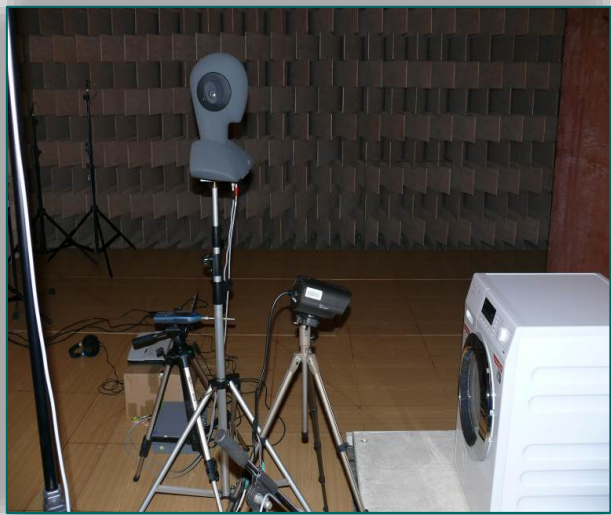
Figure 3. Binaural measurement of washing machine sound
