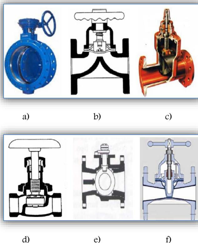
Figure 1. Different types of control valves
