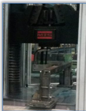
Figure 6-1: Towing assembly fixed on traction machine support
