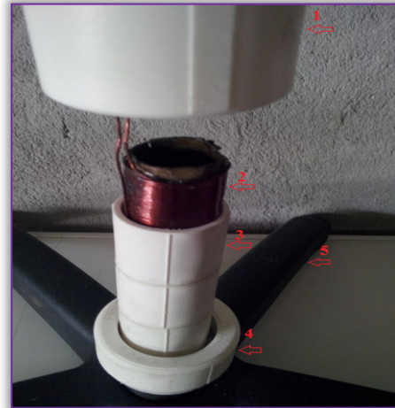
Figure 7. Assembly coil and insulation 1 = external insulation system and supportive of polypropylene ( \varphi_{int} = 52mm ); 2 = coil (140mm, d = 30mm , \varphi = 0.7 mm ); 3 = insulator system and supportive coil and from polypropylene ( \varphi_{int} = 32mm ); 4 = base supportive and fixation outer cylinder from polypropylene; 5 = base star of support cylinder and assembly seat.
