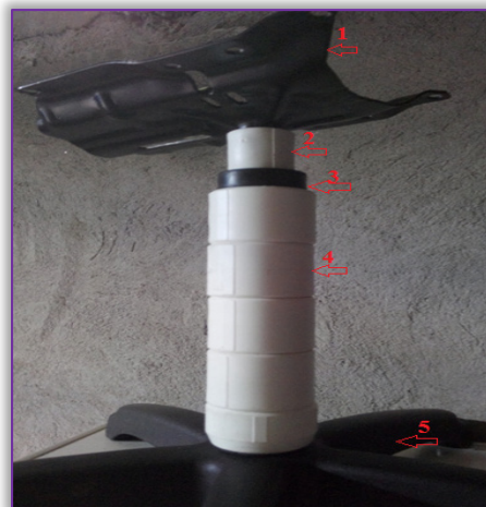
Figure 8. Assembly support of the magnetic cylinder 1 = grip and supportive seat system; 2 = limiter piston; 3 = spacer; 4 = cylinder with magnets N48; 5 = base star of support cylinder and assembly seat.
