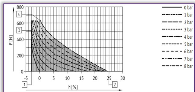
Figure 5. DMSF-10 muscle's force-contraction (relative displacement) diagram [21]
