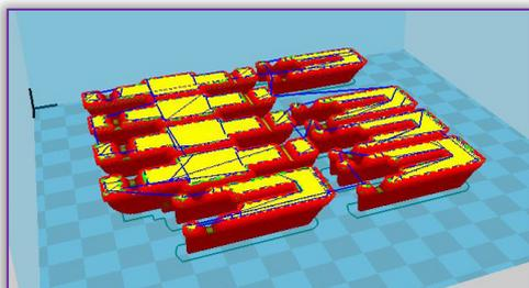
Figure 3. Fingers in the 3D printer's slicing program
