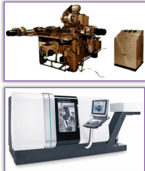
Figure 1. The first NC machine from 1951 and the most modern CNC technology
