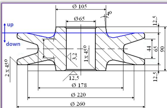
Figure 7. Sectioning of the patterns and the moulds
