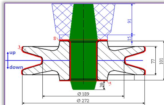
Figure 5. The dimensions of the vertical cylindrical core marks
