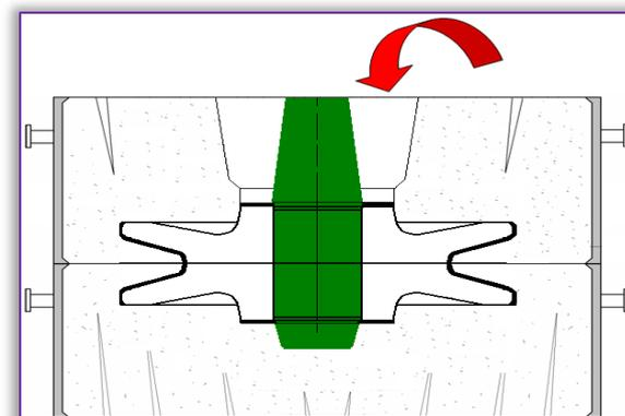
Figure 6. The mould assembled for casting
