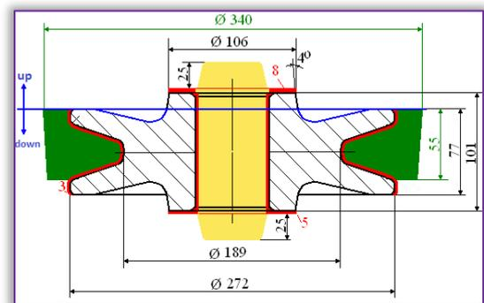
Figure 10. Establishing the manner of location of cores
