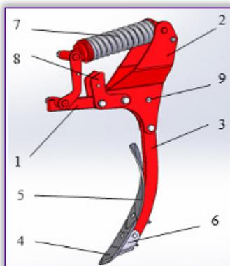
Figure 2 – Main working body of the cultivator
