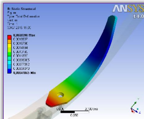
Figure 12 – Distribution of deformation on the working body wing
