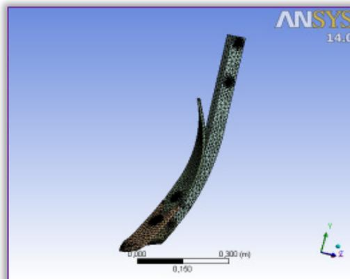
Figure 4 – Meshed model of the working body
