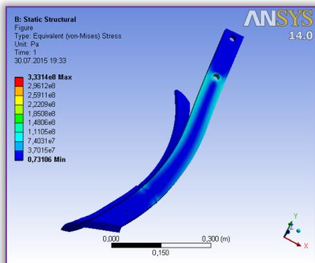
Figure 8 – Distribution of equivalent stress
