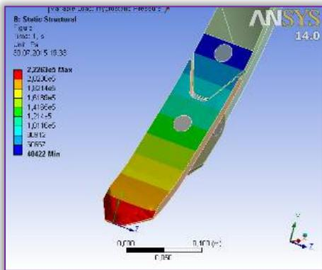
Figure 7 – Distribution of normal pressures on the working body
