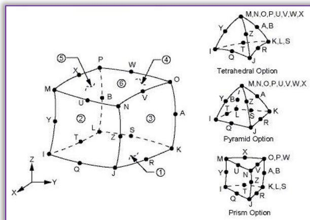
Figure 5 – Geometry of the finite element
