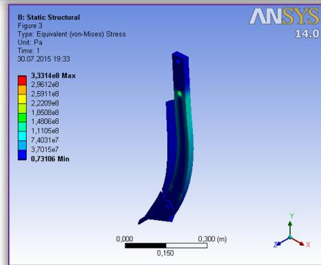
Figure 10 – Distribution of equivalent stress in the support of the working body
