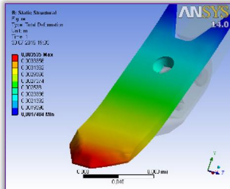
Figure 11 – Distribution of deformation on the coulters of the working body
