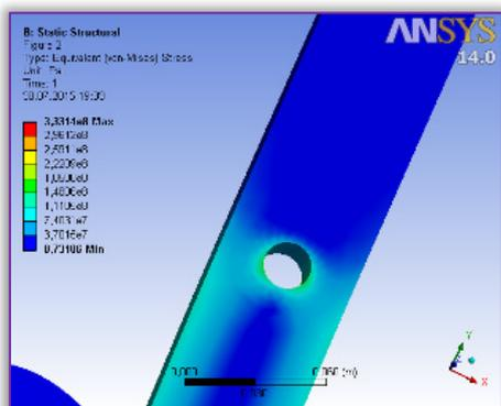
Figure 9 – Detail of the distribution of equivalent stress
