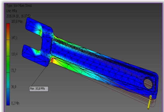
Figure 6. Maximum stresses are on the neck fixing the forks together
