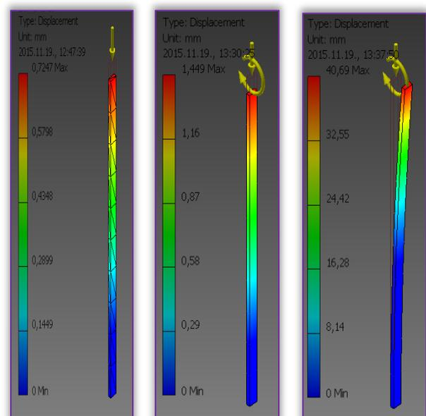
Figure 9. a. (left) Load:  $F_{\text{normal}} = 200 \text{ kN}$ , b. (middle) Load:  $F_{\text{normal}} = 400 \text{ kN}$ ,  $M = 1 \text{ kNm}$ , c. (right) Load:  $F_{\text{normal}} = 400 \text{ kN}$ ,  $M = 1000 \text{ kNm}$
