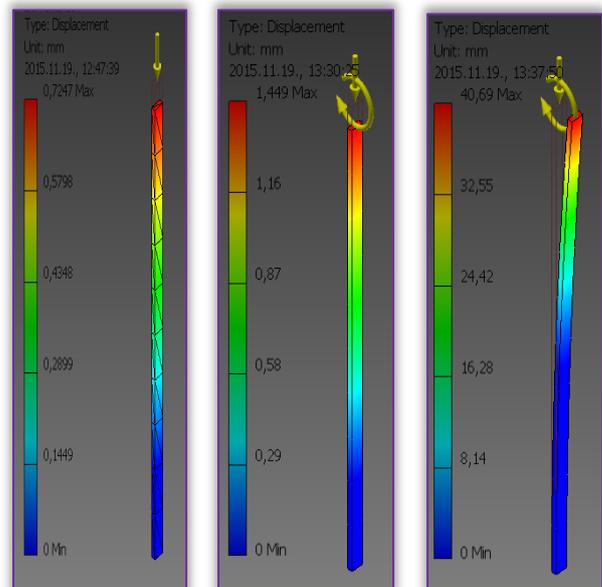
Figure 9. a. (left) Load:  $F_{\text{normal}} = 200 \text{ kN}$ , b. (middle) Load:  $F_{\text{normal}} = 400 \text{ kN}$ ,  $M = 1 \text{ kNm}$ , c. (right) Load:  $F_{\text{normal}} = 400 \text{ kN}$ ,  $M = 1000 \text{ kNm}$
