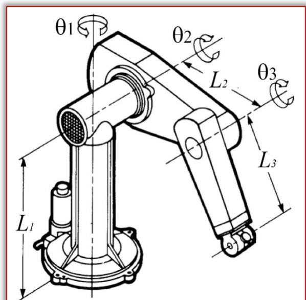
Figure 1. PUMA Robot dimensions and joint angles.
