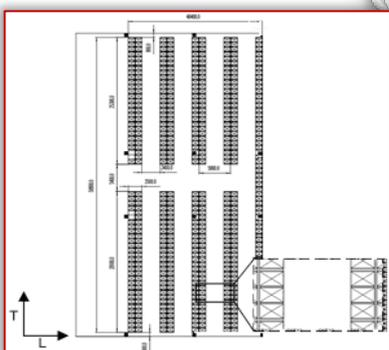
Figure 8. Wide transversal aisle (LU in longitudinal)
