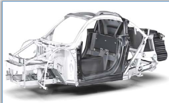
Figure 4 – Body of Audi R8 e-tron: aluminum space frame technology combined with carbon fiber components, displayed without blanking [1].
