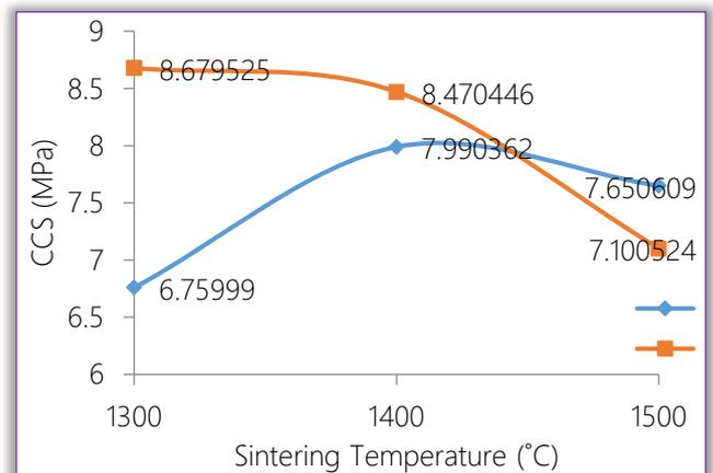
Figure 12. Effects of Sintering Temperature on the Cold Crushing Strength of Samples with varied addition of TiO<sub>2</sub>.
