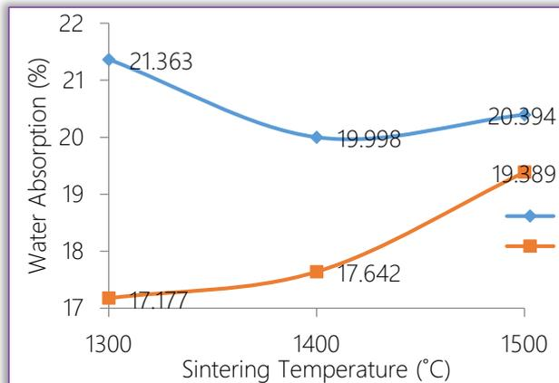
Figure 11. Effects of Sintering Temperature on the Water Absorption of Samples with varied TiO<sub>2</sub> addition.
