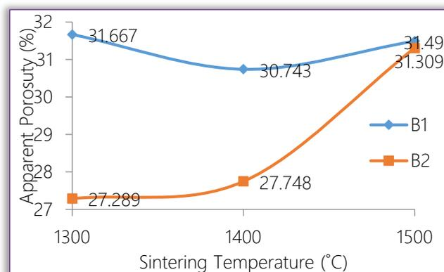
Figure 9. Effects of Sintering Temperature on Apparent Porosity of Sample with varied addition of TiO<sub>2</sub>.
