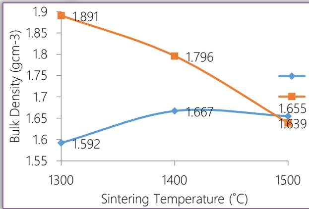
Figure 10. Effects of Sintering Temperature on the Bulk Density of Samples with varied TiO<sub>2</sub> addition.
