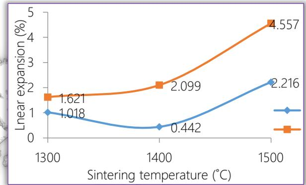
Figure 14. Effects of Sintering Temperature on the Linear Expansion of Samples with varied addition of TiO<sub>2</sub>.
