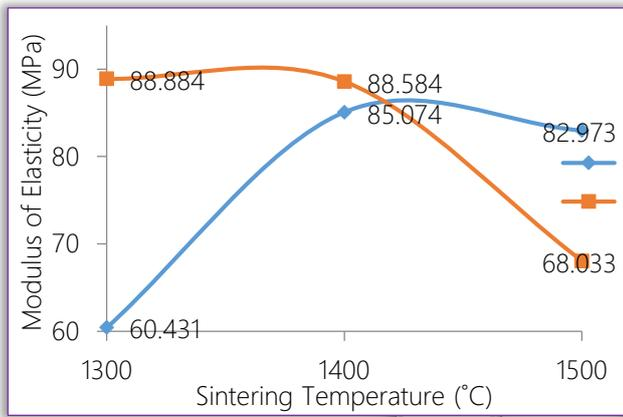
Figure 13. Effects of Sintering Temperature on the Modulus of Elasticity of Samples with varied addition of TiO<sub>2</sub>.
