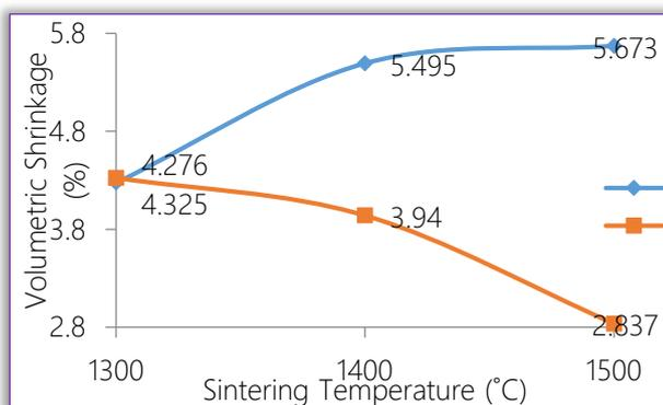
Figure 15. Effects of Sintering Temperature on Volumetric Shrinkage of Samples with varied addition of TiO<sub>2</sub>.
