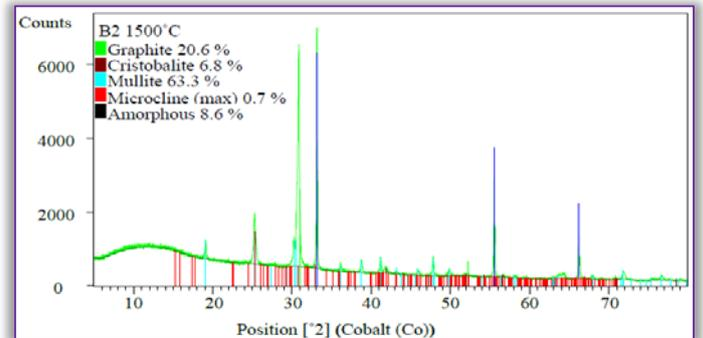
Figure 8. X-Ray Diffractometry Pattern of Sample B2 at 1500°C
