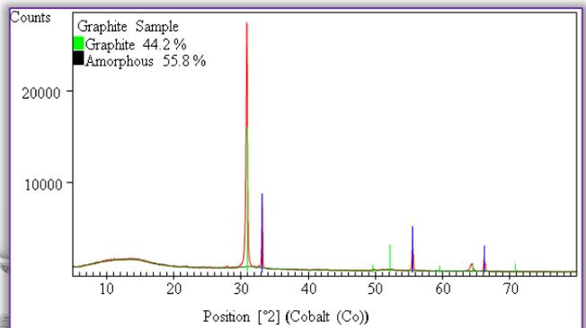
Figure 2. X-Ray Diffractometry Pattern (Phase Analysis) of graphite sample [11].
