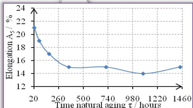
Figure 2 - Variation of elongation at break with natural aging time
