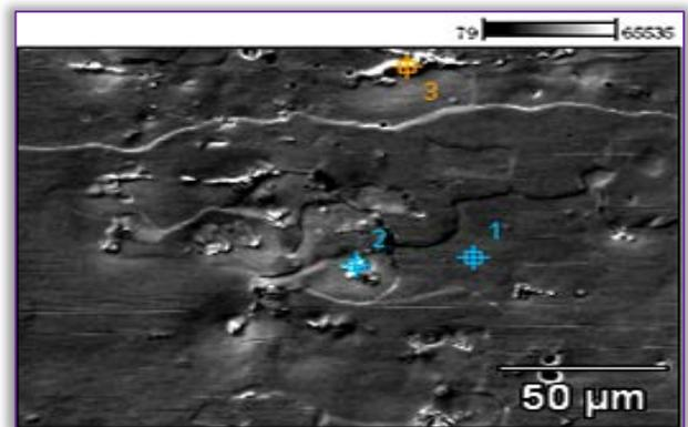
Figure 7 - Natural aging microstructure ( $\tau = 720$  / hours), 1509: 1 zoom
