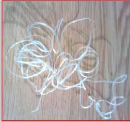
Figure 5. Measurement 5: ( a_p=1,5 mm; v_f=80 mm/min; n=600 rpm)
