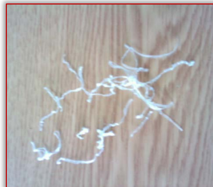
Figure 2. Measurement 2: ( a_p=2 mm; v_f=80 mm/min; n=1200 rpm)
