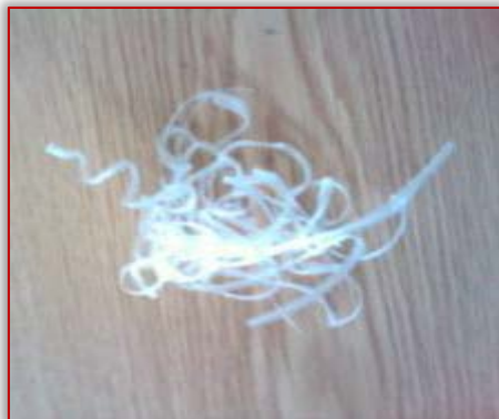
Figure 1. Measurement 1: ( a_p=2 mm; v_f=80 mm/min; n=600 rpm)
