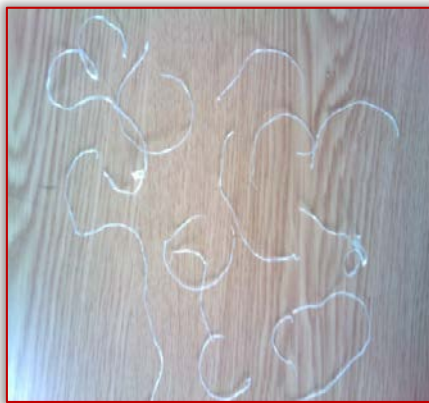
Figure 6. Measurement 6: ( a_p=1,5 mm; v_f=80 mm/min; n=1200 rpm)
