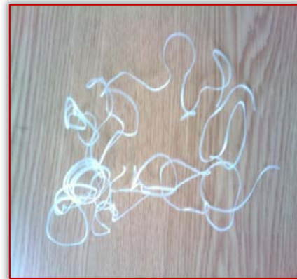
Figure 8. Measurement 8: ( a_p=1,5 mm; v_f=300 mm/min; n=1200 rpm)
