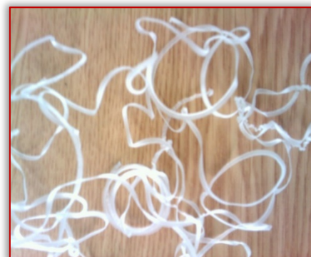
Figure 4. Measurement 4: ( a_p=2 mm; v_f=300 mm/min; n=1200 rpm)
