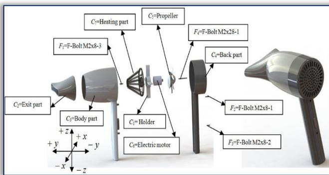
Figure 2. Exploded view and assembly of hair-dryer
