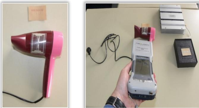
Figure 4. Placement of RFID tag and tag reading
