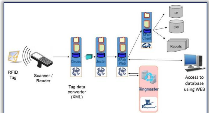
Figure 3. Diagram of the RFID software system architecture
