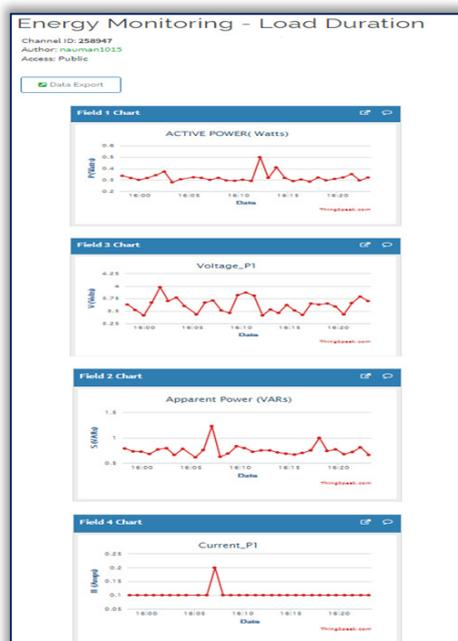
Figure 17. GUI for online energy monitoring
