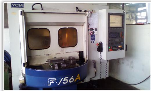
Figure 7. CNC Milling machine [8]
