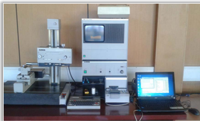
Figure 2. Surface roughness measurement system Talysurf-6 connected with computer
