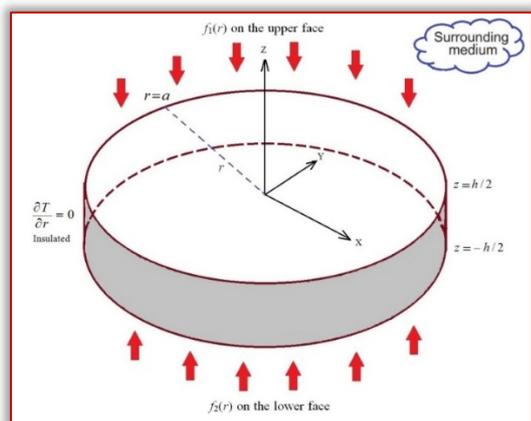
Figure 1. Plate physical configuration
